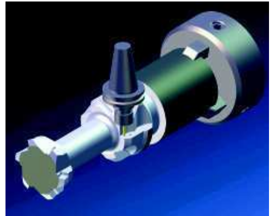
Millturn: Machining in a lathe with C-, Y- and B-axis
